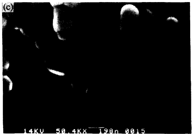
Fig. 22. Electron micrograph of Cookson Entek polyethylene separator: (a) 5.04 KX; (b) 10.2 KX; (c) 50.4 KX.
